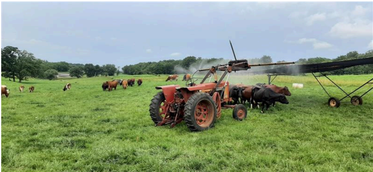
Pasture mister with mobile shade (built on an old hay elevator frame using shade cloth. Designed by Kevan Jahnke, Organic Valley Cooperative.
